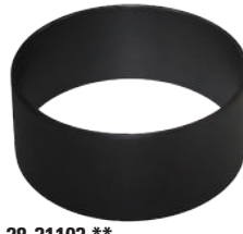
28-31103 ** I.D. 161mm, O.D. 169mm Height: 73.3mm **Fits WSM# 003-504 housing or other aftermarket housings w/replaceable wear rings
