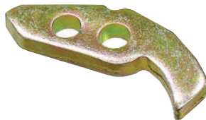
740-7022 Thickness: 6mm. Holes I.D: 8.3mm & 7.5mm Same Pawl in Part No. 740-7023 & 740-7024
