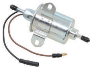
66-40001 In-Line Fuel Pump Volt-12V, Max Pressure: 8lbs. Pipe O.D.: 6.6mm. Wire(L): 70mm. Bolt Hole: 7 X 9.6mm
